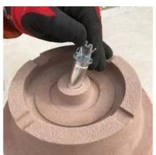
Insert the starter into the hole in the lid of the crucible.
