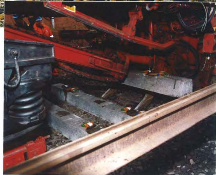
Above: Modified Fairmont Tamer P8-11 track laying machine.
