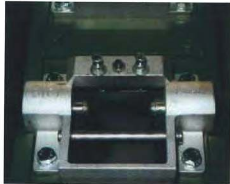
Detail of an EVOLUZIONE locking system seen from the bottom of the mould.
