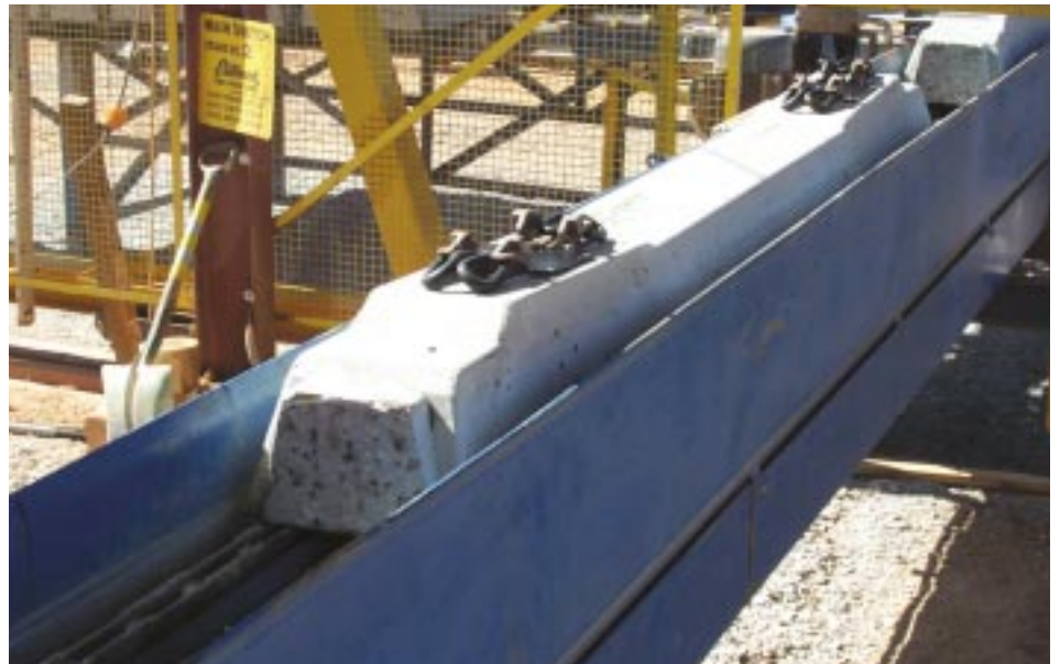
Concrete Sleeper pre-assembled with FASTCLIP fastenings
