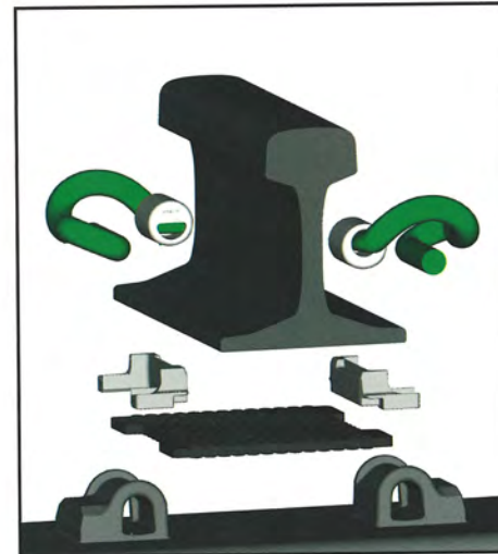
▲ Exploded view of the e-PLUS system showing the separated Toe and Sidepost Insulator.
