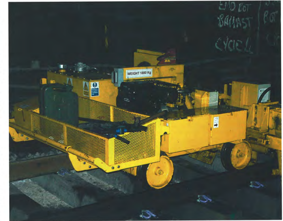
▲ Pandrol MK4 clip application machine, capable of installation and extraction.
