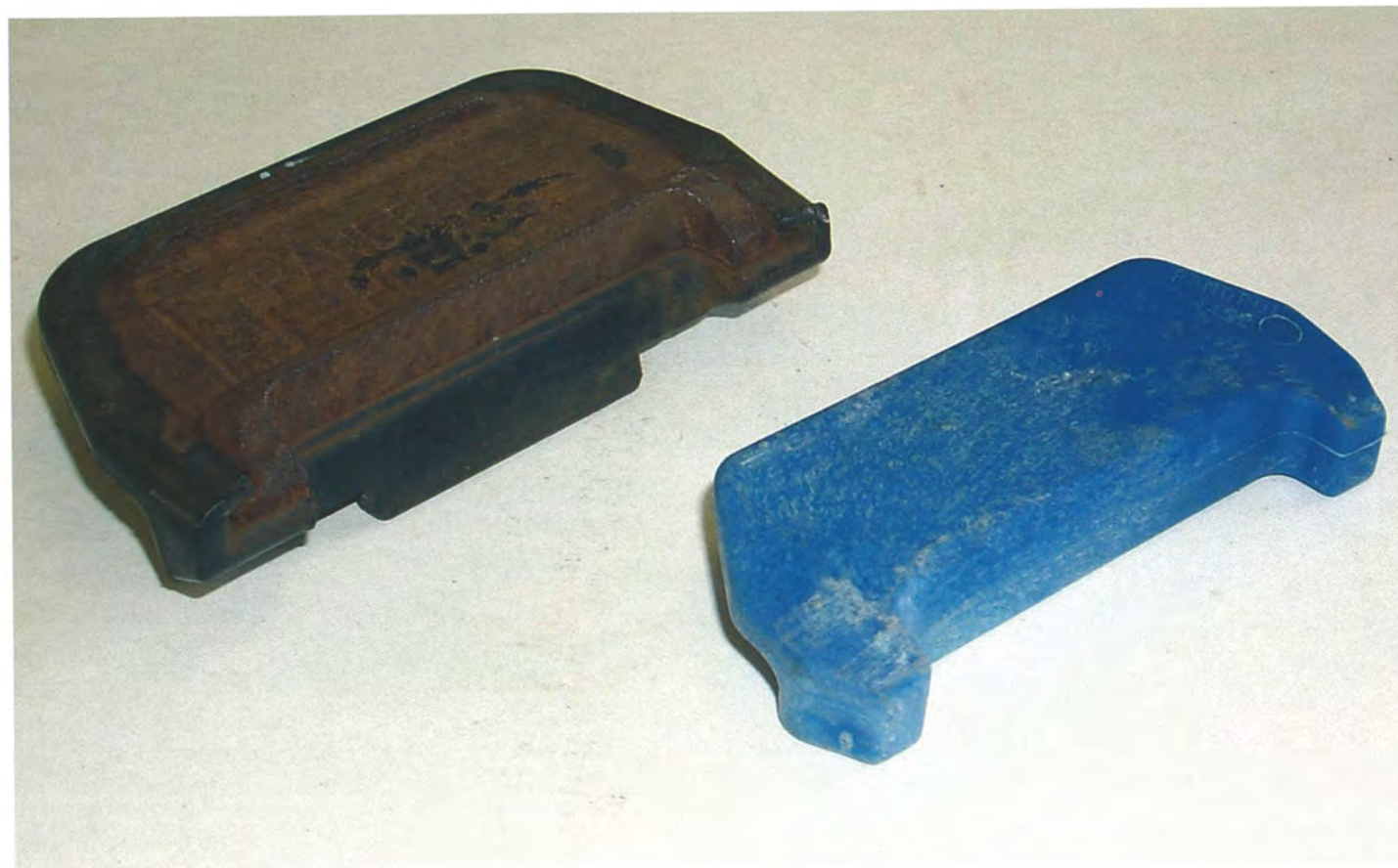
▲ A Heavy Duty HD8 Insulator for 30T axles (black) shown against a Standard 4452 Insulator for 25T axles (blue).
