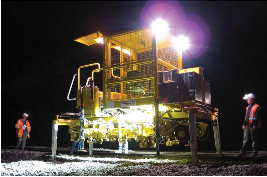
Rosenqvist CD500 hi-output clipping machine for Fastclip
