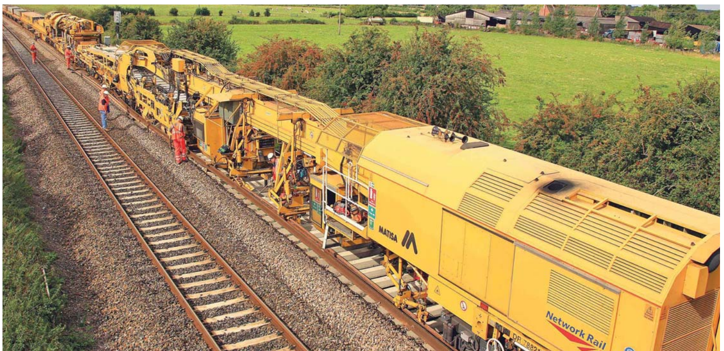
Track Renewal Train working on Network Rail
