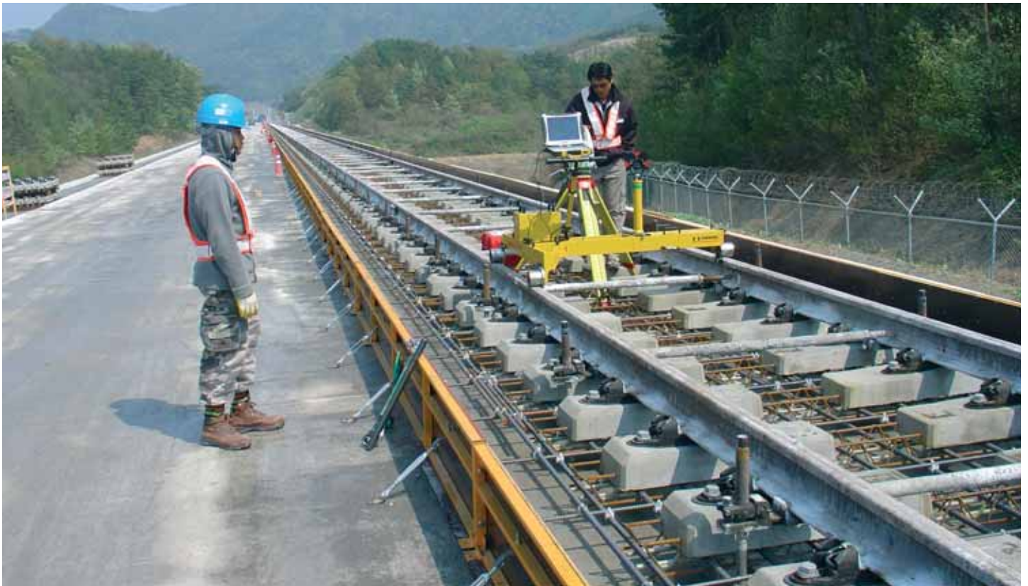
Measurement of track geometry
