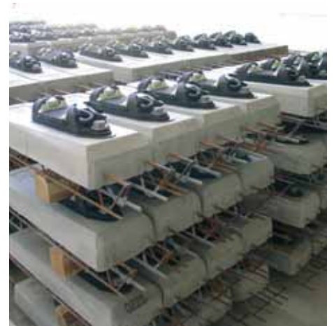
Loading manufactured concrete sleepers pre assembled with the Pandrol SFC system
