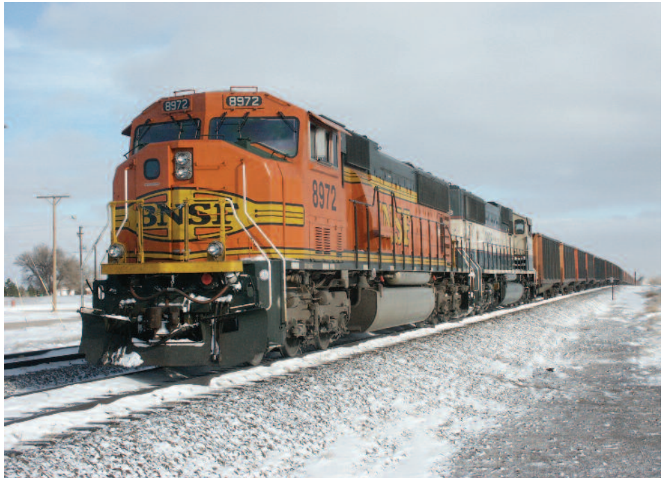
Low rail temperatures and wheel damage present a large risk of rail breaks
