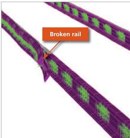
Figure 2 Broken rail simulation
