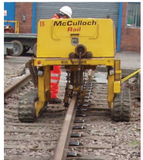
Rail threading is easier thanks to the curved pad
