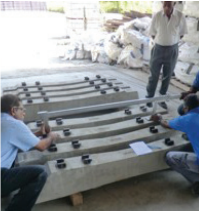
Finished Pandrol Fastclip FE sleepers being checked at the Mastrack factory
