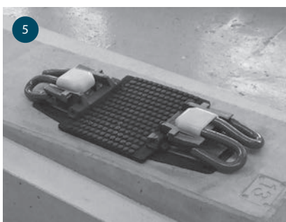
5 Pandrol Fastclip fastenings are installed into the parked position. The finished concrete elements would normally be delivered to the construction site in this configuration.
