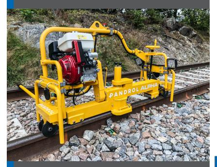
A robust rail profile grinder that is easy to use and grind the complete profile in one operation.
