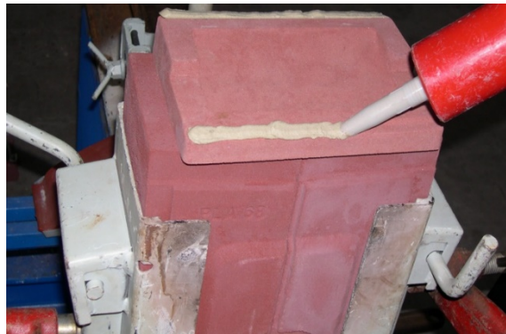
Figure 37: Apply cartridge luting paste
