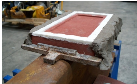
Figure 57: Pate A Lute after cutting
