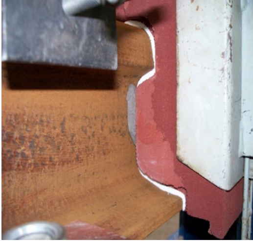
Figure 52: Paste applied in the luting strip
