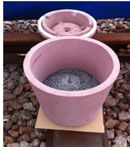
Figure 18: Crucible Ready for Use
