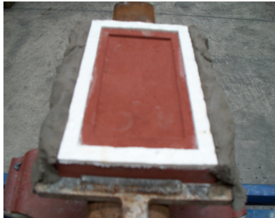
Figure 56: Pate A Lute before cutting and levelling
