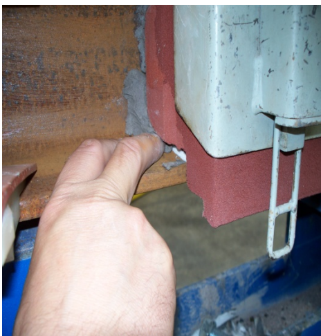
Figure 54: Make sure that the Pate A Lute is in contact with the felt
