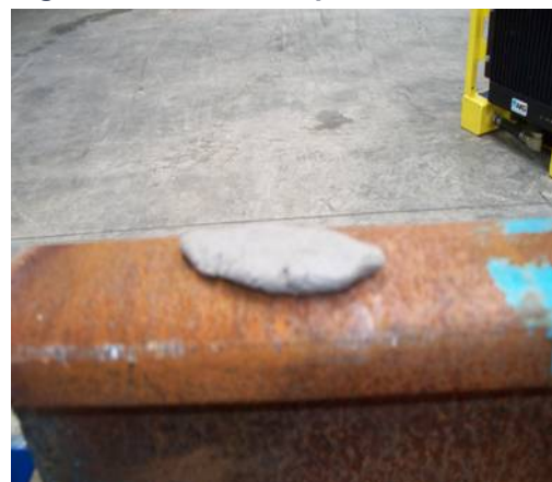
Figure 51: Flattened piece of 35 mm Pate A Lute
