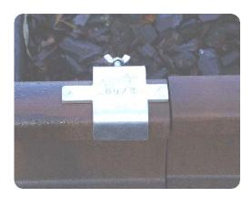
▶ Position the support arm in contact with the gauge lug so that the rail saw fastening pin is on the gauge side and then tighten up the clamp as tightly as possible.
