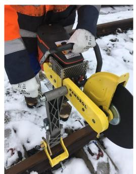
The double input socket enables the rail saw to be positioned either on the inside or the outside of the track.
