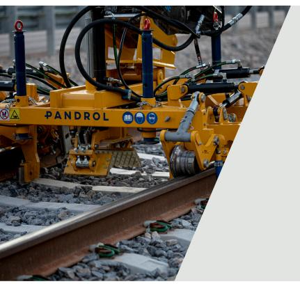
Clip Driver CD300 IQ is a high-production clipping machine designed to install Pandrol Fastclip FC and FE fastening systems.
