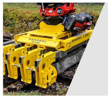
Pandrol's range of carrier-mounted Sleeper Layers achieve fast, accurate sleeper laying and spreading, with an easily adjustable tool designed to fit most kinds of sleepers. The SL400 can handle four sleepers simultaneously, while the SL850 can handle up to eight at a time.
