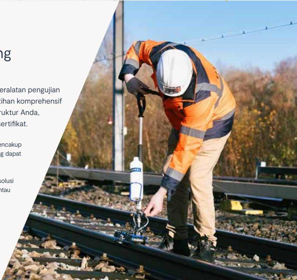
Ultrasonic Testing device
