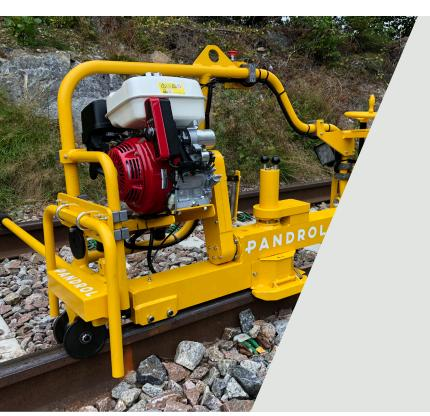
Pandrol's rail equipment products encompass market leading solutions for welding kits and track mounted machinery. The Alpha Grinder extends the life of the track by grinding the complete profile in one operation, delivering the ergonomic design and precision efficiencies that Pandrol are renowned for.
