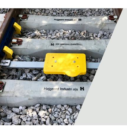
The Pandrol Clamp Beam Balise Mounting System (BMS) is used to install balises (transponders) into track securely and efficiently.
