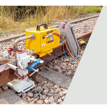
The Pandrol High Flow Preheater (HFP) is a universal preheating system for use when welding on site. It has been designed to replace the need for most existing equipment currently used to raise the temperature of the parent steel before welding.
