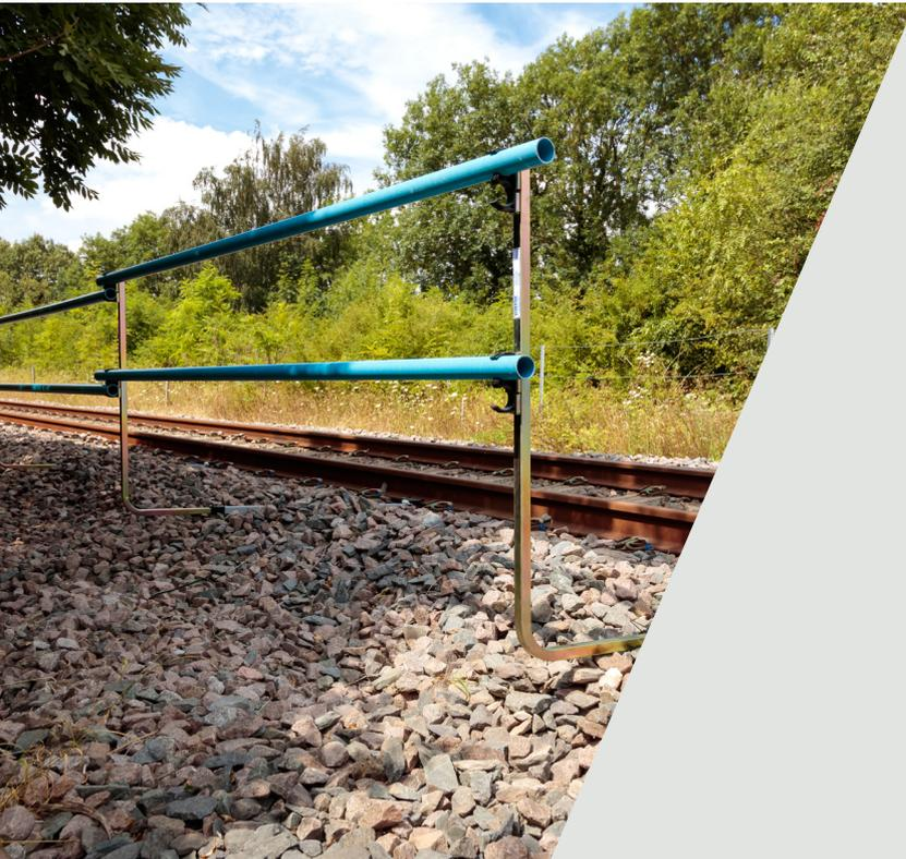
The Telescopic Safety Barrier is a quick and easy-to-install barrier that creates a safe zone for track work, separating people from the live traffic area. It is clamped to the rail foot of the live traffic line and has been engineered for varying line speeds. It also has insulation properties, giving protection in overhead line and third rail environments.
