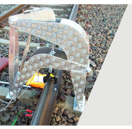
Reducing the risk of derailment as a result of track buckles or rail breaks has long been a priority for railway companies and track engineers. Measuring the stress-free temperature of continuously welded rail is a key part of this, enabling weaknesses and risks to be identified and managed. In the past this was a time-consuming, expensive and often unreliable process that involved cutting the rail.
