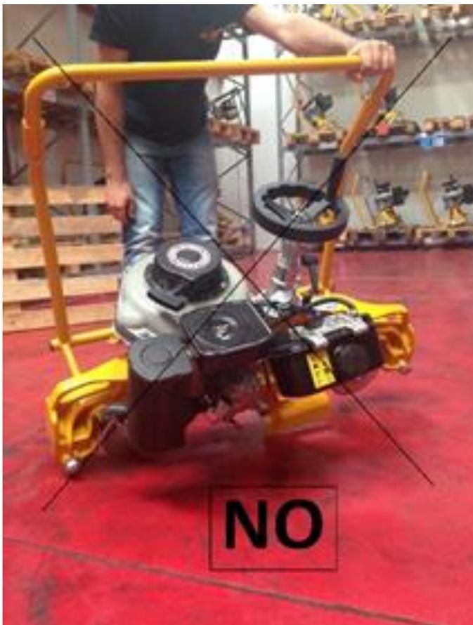
**Figure 13: Tilting operation**
