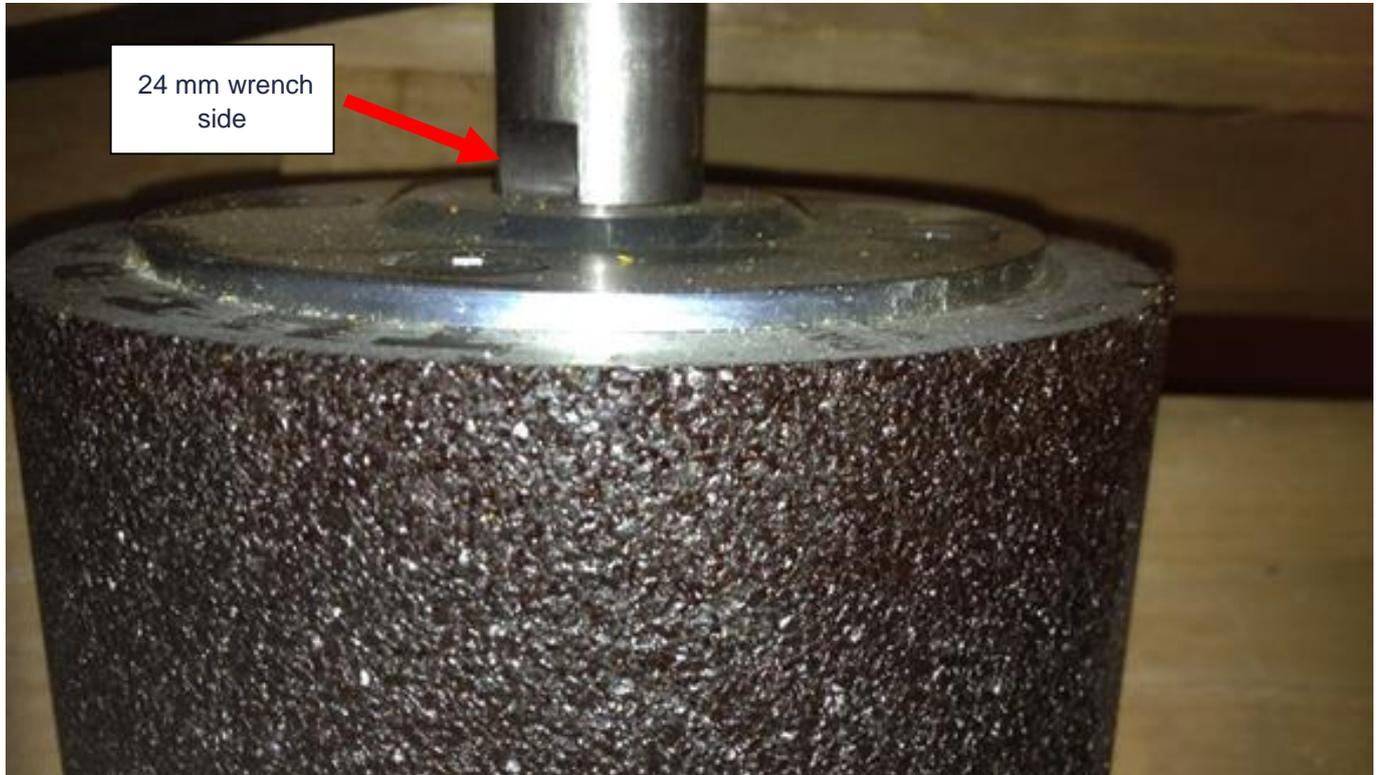
should be run at midrange rpm.
