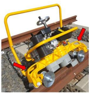
Figure 6: Lifting points
