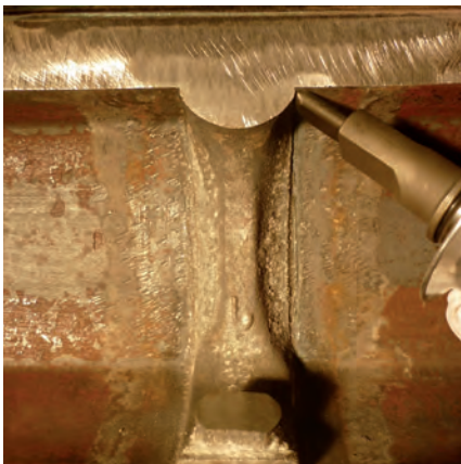
Web/head connection hammering.
