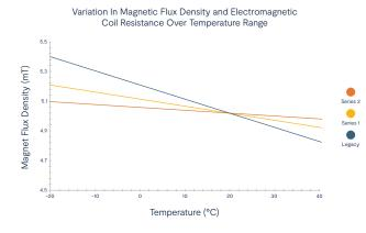
The change in magnet material reduces variation in magnetic flux density with temperature:
