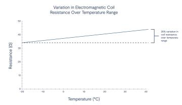
We control coil current to ensure a consistent magnetic field across the full range of supply voltages and operating temperatures. On legacy products, the magnetic field can vary by as much as 38%.
