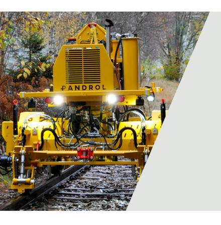
The CD400SP IQ is our second generation walk-behind clipping machine, following the original reliable CD400SP.
