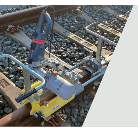
The Monobloc Electrical Weld Shear EME1/EME2 is an electrical rail shearing machine designed to shear off the red-hot metal remaining around the rail head after aluminothermic welding of Vignole rails. During aluminothermic welding, a deadhead of excess metal remains above the rail head. This was traditionally removed manually with a hammer and chisel. The Monobloc Electrical Weld Shear automates this process and removes the risk of damaging the rail.
