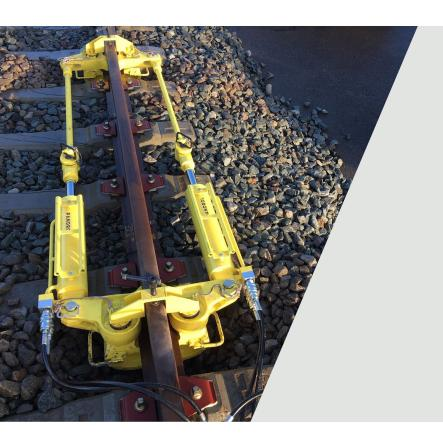
The Rail Stressor TR75 has been designed for the stress relief or replacement of continuous welded rails (CWRs). It is used during maintenance works to stretch long welded rails before aluminothermic welding and to secure the tensioned rail while cutting. It is capable of joining and maintaining a constant gap between the two rail ends.
