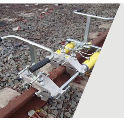
The Bi-Bloc Weld Shear EGH1/EGH2/EGH2 RAG are hydraulic rail shearing machines designed to shear off excess metal after aluminothermic welding of Vignole rails (EGH1/EGH2) or grooved rail (EGH2 RAG). During aluminothermic welding, excess metal remains above the rail head. This was traditionally removed manually with a hammer and chisel. The Bi-Bloc Weld Shears automate this process and remove the risk of damaging the rail.
