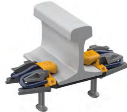
Fastclip is a total system in which all components are delivered to site pre-assembled on the sleeper or baseplate. Once the sleepers are laid and the rail installed the clip is simply pushed onto the rail by means of a simple drive action.
