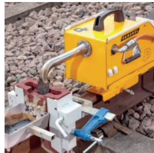
Perform secure and safe welding thanks to the HFP preheater.
