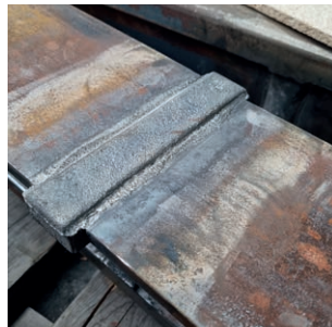
Eliminating discontinuity under rail foot.
