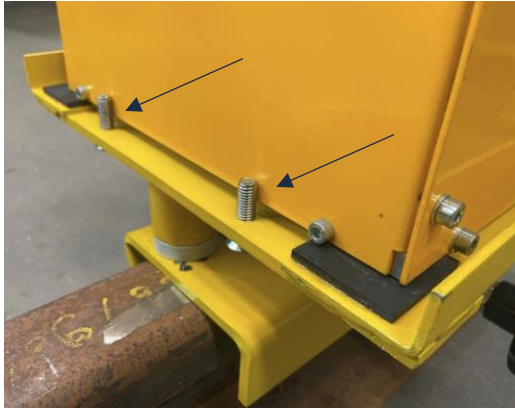
Support with retaining screws in operating position
