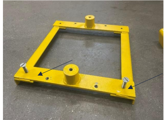
Support with retaining screws in storage position
