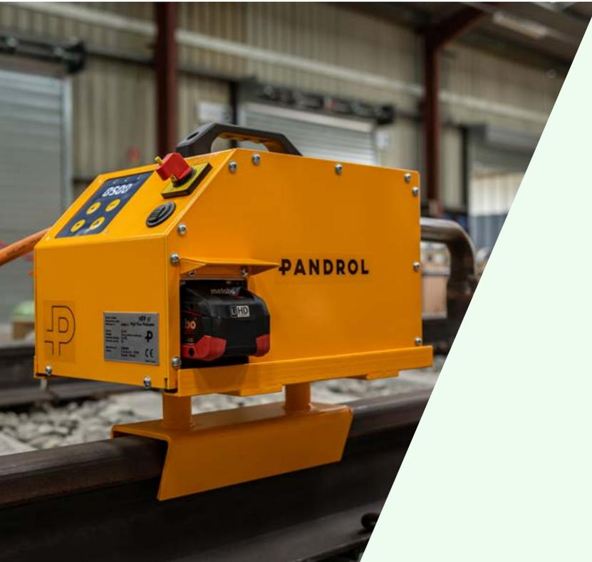
The HFP 36V is battery powered and fully automated for easier, more reliable operation: the ignition, timing and stop require no manual interference or flame adjustment. It uses only propane, no oxygen is required, reducing costs and reducing the total weight to carry on site.
