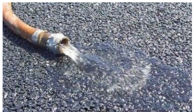
Figure 11: Granular structure of Pandrol RBR makes it water permeable
