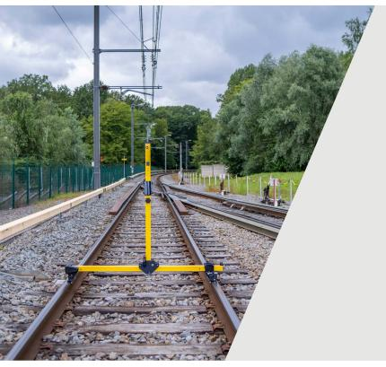
The Data Logging Laser Height and Stagger Gauge (P8000) is a development of the P4640 model, which uses laser technology to take measurements and check the overhead contact wire is correctly positioned. In the Data Logging version, the user is able to log and store data directly to an Android phone, either by using the equipment as a digital recording gauge or in conjunction with a downloadable app.
