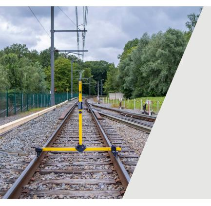
The Laser Height and Stagger Gauge (P8100) uses laser technology to enable the user to take measurements of the height and stagger of overhead catenary wire (OHL) quickly and accurately, from a standing position. Super elevation (SE) and rail edge to face of structure (REFOS) can also be measured.
