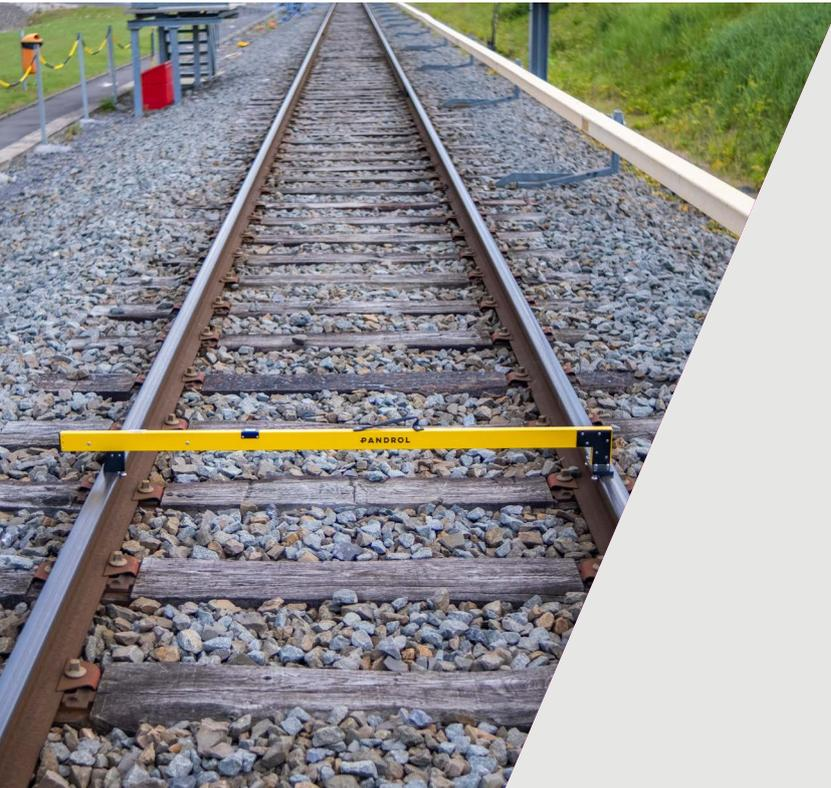
The P-Way Gauge (P5000) is a reliable, accurate track gauge suitable for use in all aspects of rail engineering to measure track gauge and super-elevation.
