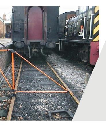
Pandrol's Platform Gauge (P4050) is primarily used by inspectors to assess the positioning of station platforms. It enables a single operator to take measurements from the platform, without track possession. The gauge's open frame allows the operator to lower the tool onto the track from the platform and move it quickly should a train approach.
