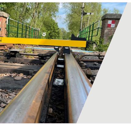
The Switch and Crossing Confirmation Gauge (P4670) has been specifically designed to carry out dimensional checks within the moveable part of a switch unit. The gauge measures free-wheel clearance (the distance between the running edge of the stock rail and the rear face of the adjacent switch rail), free-wheel passage (the distance between the rear face of an open switch and the running edge of the closed switch) and the switch rail wear profile.
