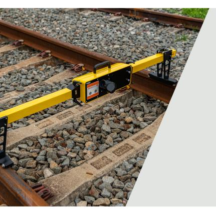
The RouteScan (P5650) gauge uses 2D laser scanning technology to take quick, accurate structure clearance measurements in relation to the permanent way. It can be used to take measurements of tunnels, bridges, platforms, datum plates, signals, rail positions, and overhead line catenary wire position.
