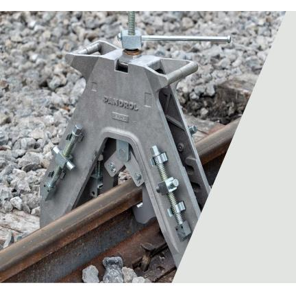
The A-Frame Rail Aligner ensures the precise alignment of rails before aluminothermic welding and holds them in position throughout the welding operation. In doing so, it increases the operator's safety, as well as ensuring perfect weld geometry.
