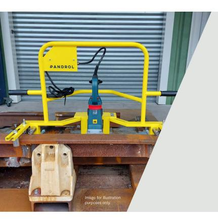
The Pandrol Precision-Grinder E-115-GDR is designed to grind aluminothermic welds made on guide rails with precision and ease. The ergonomic machine is self-supported on the rail thanks to its six insulated rollers. Its flexible design allows the user to adjust the grinder in any direction with ease.
