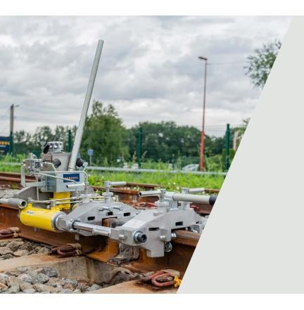
Pandrol's Weld Shear Hand Pump (EPM2) is a manual shearing machine designed to shear off excess metal after aluminothermic welding.
