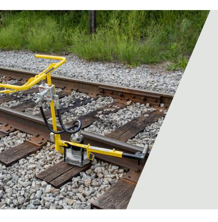
Pandrol's Multi-Purpose Grinder (06950-TST) is a versatile tool that is suitable for a wide range of field weld grinding operations.
