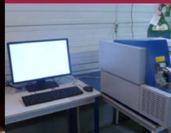
Chemical analyzes with spectrometer
