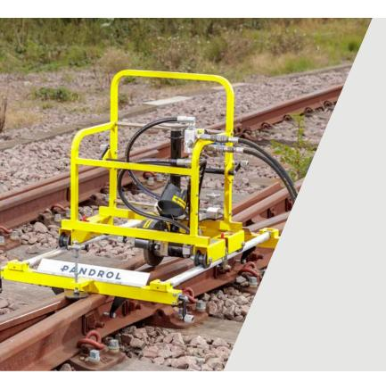
Pandrol's Precision Frog Grinder (09200A) is a hydraulic-powered, track-mounted machine that brings detailed, four-axis grinding to the field.
