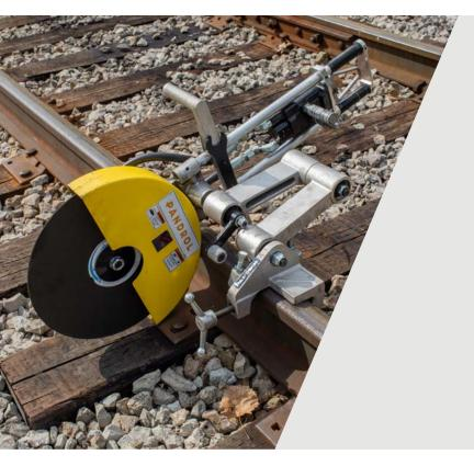
Pandrol's Reversing Rail Saw (03900A) is a hydraulic-powered abrasive rail saw that can cut rail safely from either side. The saw simply needs to be pivoted to the other side of the rail – there is no need for disconnection or realignment. Sparks are safely directed downward, no matter which side of the rail the operator is cutting from.
