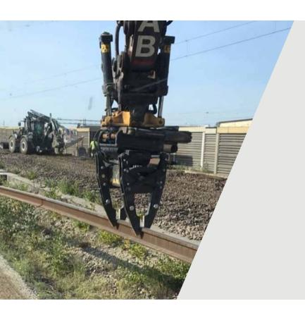
Pandrol's Sleeper Grabber SG60 is a high-performance tool for heavy-lifting track procedures.
