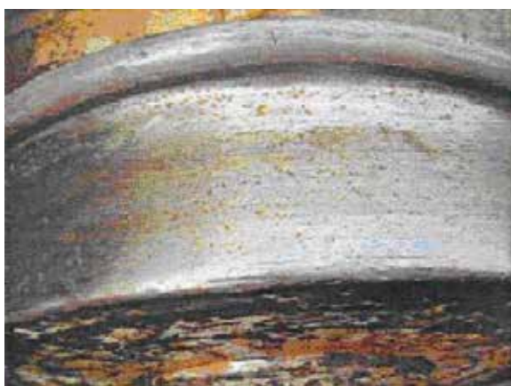
Figure 160. Circumferential cracking limit associated with rollover
