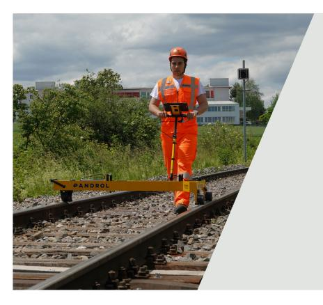
Developed in partnership with Amberg Technologies, Pandrol's GeoVizio-TR-Smart is a new smart track geometry trolley for measuring the quality of track.
