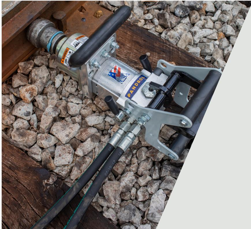
Pandrol's Impact Wrench (02500) is a rugged hydraulic tool that can handle the toughest of jobs, including removing and tightening crossing, frog and track bolts.
