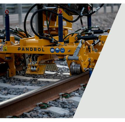
Clip Driver CD300 IQ is a high-production clipping machine designed to install Pandrol Fastclip FC and FE fastening systems. Clip Driver CD300 IQ is a version specially designed for e-Clip fastening system.
